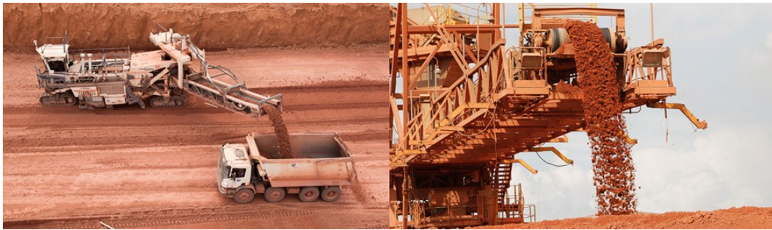
Figure 1. Bauxite extraction operation at Paragominas: strip and stack mining process.
